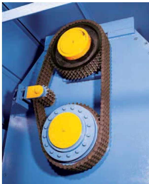
上滾軸以滑動離合器來驅動 Top Roll Is Actuated With Slip Clutch
