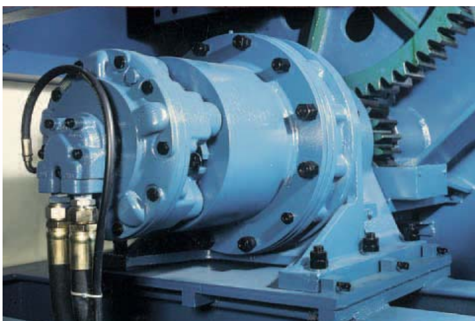
低速徑向活油壓馬達和傳動速機 Low Speed Radial Piston Hydraulic Motor And Speed Reducer.
